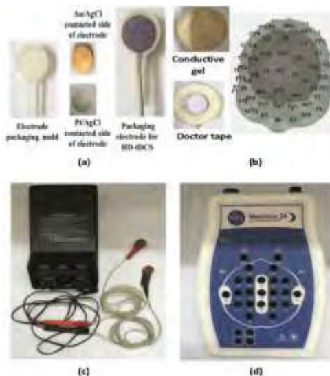
Figure 1. (a) Fabricated electrode mould and packaging (b) Positioning fabricated electrode on interested region of brain with conductive gel and doctors' tape (c) Fabricated electrode made compatible with tDCS device (d) Fabricated electrode made compatible with RMS EEG device.
