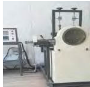
Figure 04: Pelton wheel Turbine
