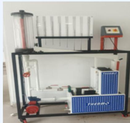
**Name of the Equipment-08:** Orifice And Mouthpiece Apparatus
