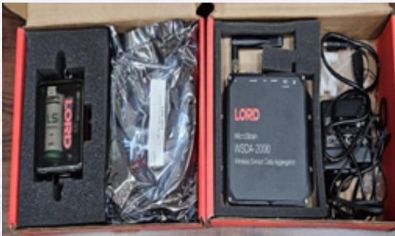
**Name of the Equipment -13:** Three Channel Analog Input Sensor with 14 pin connectors
