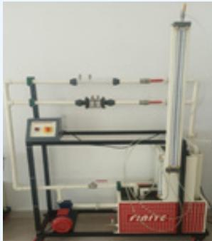
**Name of the Equipment-06:** Venturimeter & Orificemeter
