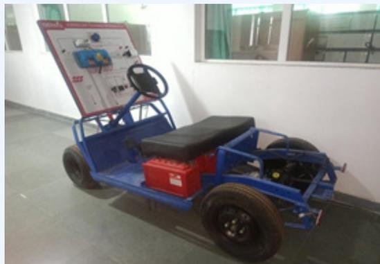
The 4-Wheeler Electric Vehicle Training Working Model is a practical, hands-on training tool designed to teach individuals about electric vehicles (EVs) specifically focusing on 4-wheeler EVs. It is essentially a scaled-down version of a real 4-wheeler EV, complete with a motor, battery, charging system, and other components.
