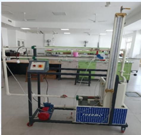
**Name of the Equipment-17:** Losses due to friction in pipe
