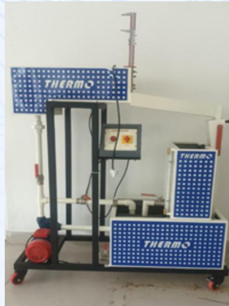
**Name of the Equipment-07:** Discharge Over Notches
