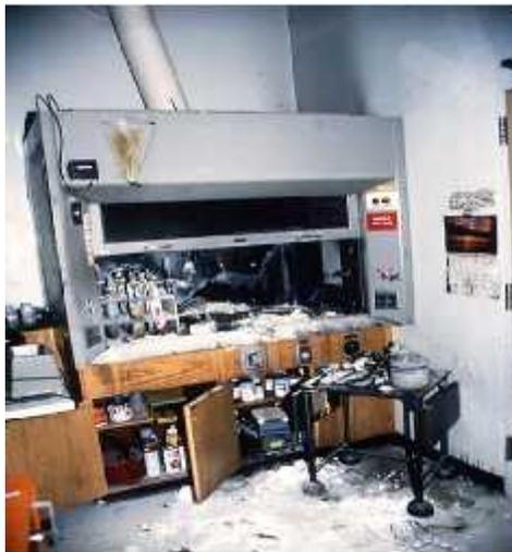
*A researcher was involved in a chemical explosion in the UCSB Chemistry building. He inappropriately mixed a strong oxidizing acid (nitric acid) with organic solvents inside a waste container within a fume hood.*
